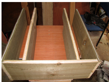
11. Run a line of wood glue along the edges of the walls and base.
