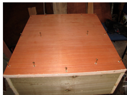
12. Position the front panel and fix firmly with screws.
