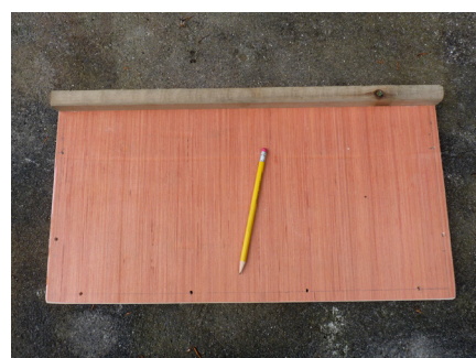
15. Screw the rear batten to the underside of the lid.
